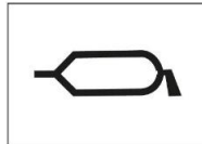
Figure 25. Lubrication places marked on the Baler
