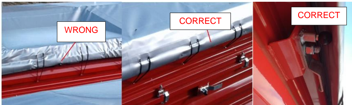
Figure 3. Correct tensioning of the tarpaulin cover
