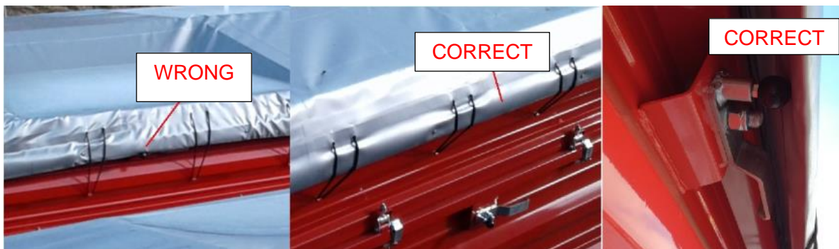
Figure 3. Correct tensioning of the tarpaulin cover
