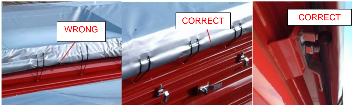
Figure 4. Correct tensioning of the tarpaulin cover
