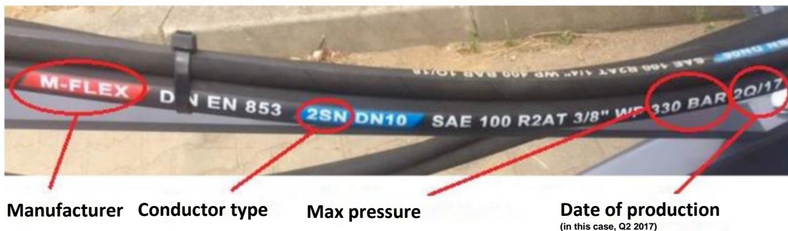
Fig. 21. Marking of the hydraulic lines
