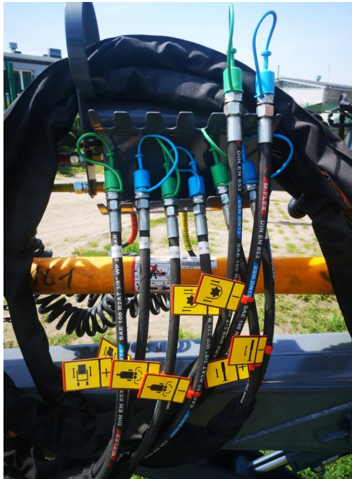
Fig. 22. Pictograms on the hydraulic connectors for easier connection to the tractor (standard)
