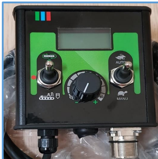
Fig. 26. Control panel for adjusting the speed of the floor conveyor by means of a potentiometer – control knob (optional accessory).
