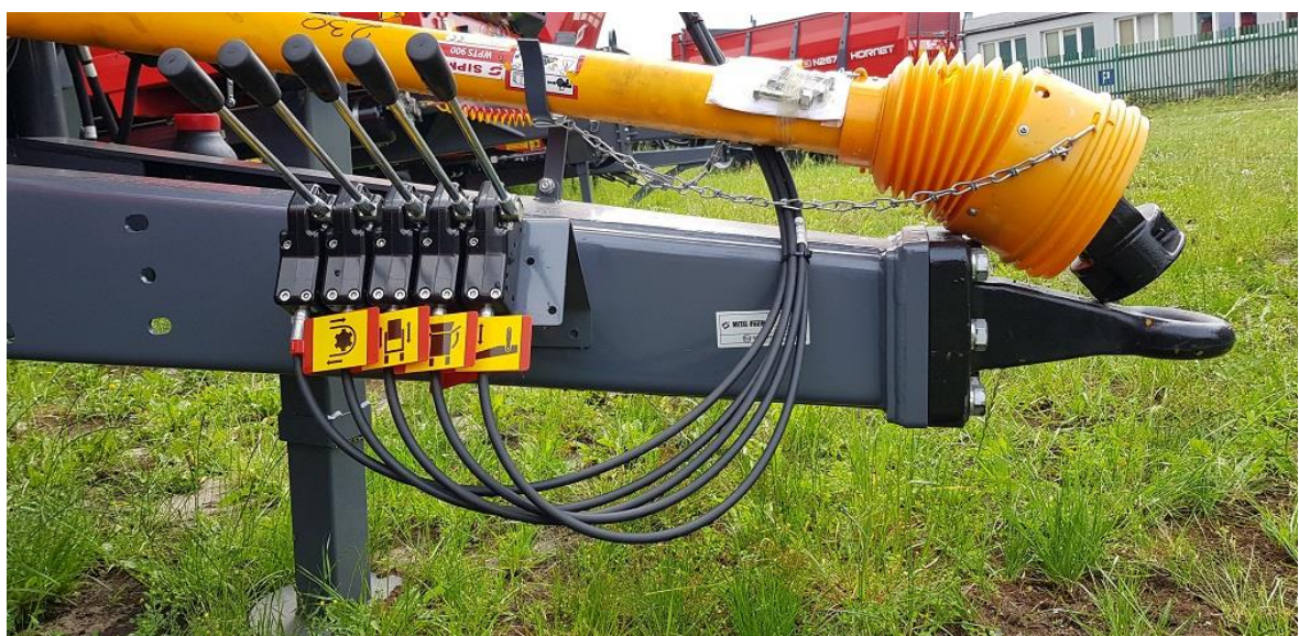
Fig. 23. Pictograms for the control levers of the distributor (distributor control is optional)
