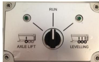
Figure 11. Suspension control panel
