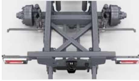
Cross braces in the rear part of the frame - reinforcement for the tipping axis.
