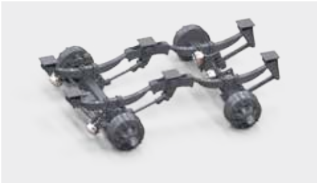
Tandem suspension with a 4-leaf spring.
