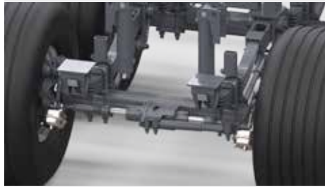
Two passive swivel axles (1 and 3) with a 120mm beam.
