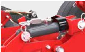
Hydraulic depth adjustment - ensures precise depth adjustment
