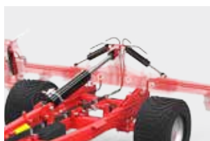
Hydraulic adjustment of operation through U910 carrier
