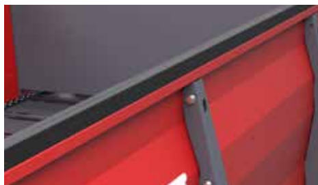
Sides protected by rubber strips to prevent damage
