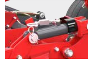
Hydraulic depth adjustment - ensures precise depth adjustment
