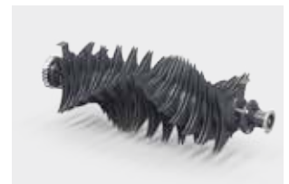
Four-blade cutting rotor, V-shaped - Cutting length 77mm, 15 cutting knives individually protected by springs.
