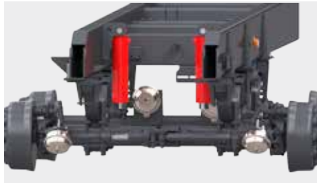
Hydraulic axle stabilization.
