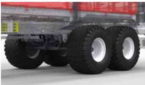
Wheels 500/50-17" - ensure better stability and traction on various types of terrain
