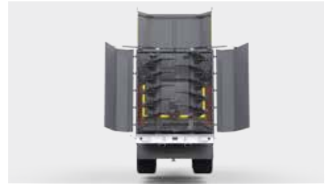
The ability to convert the trailer into a spreader after installing a vertical adapter
