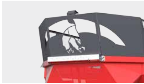
Slide position indicator - enables precise control over the slide's setting, enhancing work efficiency
