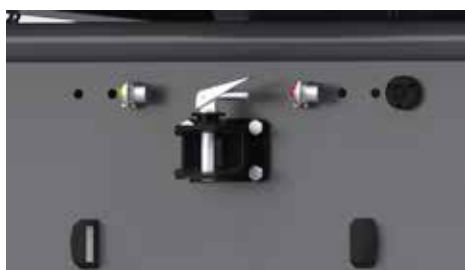
Media - hydraulics and electrical connections for the second trailer.
