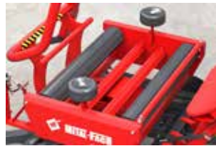
Rotary table - The design with four rotating shafts prevents bales from slipping during wrapping
