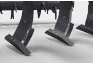
Rotary coulters blades with the Michel system. Working depth of up to 40cm.
