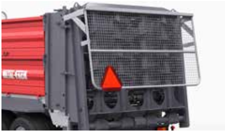
Adapter cover automatically lifted when raising the rear wall (slide)
