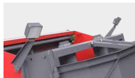
Work lights for nighttime operation - spotlights
