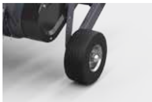
Copying wheel - reduces the pressure of the pickup on the ground, allowing easy height adjustment (10 settings)
