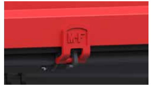
MF-branded hinges - allow for easy opening and closing of the side walls, facilitating the loading and unloading of materials
