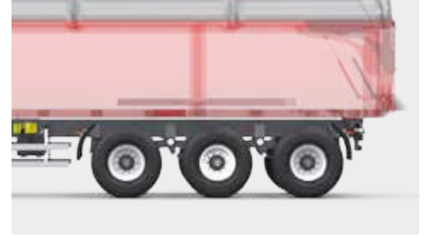
Three-axle suspension - TRIDEM with a 4-leaf spring.
