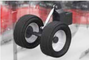
Double support wheels for maintaining precise working depth
