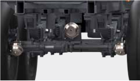
Hydraulic stabilization on the third axle.
