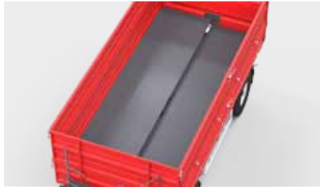
A floor made from two pieces of material allows for greater machine rigidity.
