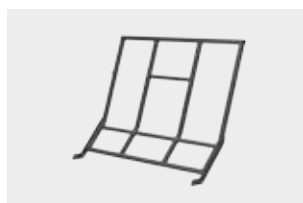
The altered shape of the wall allows for an increased number of loaded bales
