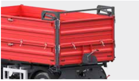
Hydraulically closed rear wall
