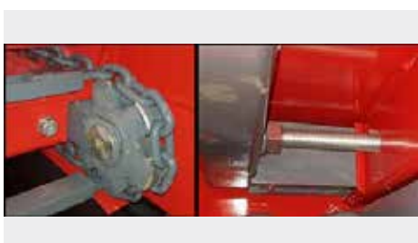
Chain tensioning - - Properly tensioned chains reduce the risk of chain slack, which can lead to accidents, chain derailment, or equipment damage.
