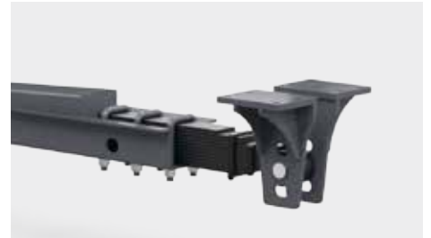
Hydraulically cushioned drawbar - reduces vibrations, improving ride comfort and enhancing safety
