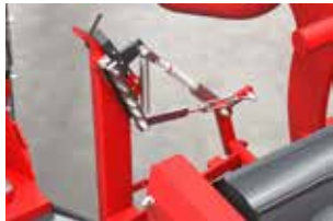
Film cutting - operates automatically after the completion of bale wrapping."
