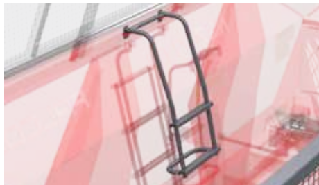
Possibility to mount a ladder inside the shell (spreader)
