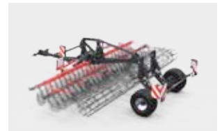
Trolley for the soil cultivation and seeding unit for versions above 4.5m
