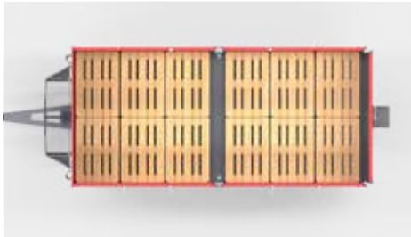
The length of the cargo space is 5385mm. The pallet width is 2410mm. It can accommodate 12 Euro pallets.
