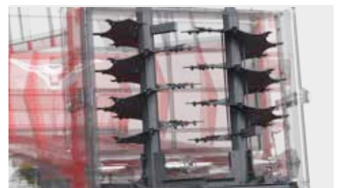
Adapter - blades of elevated durability made from HARDOX
