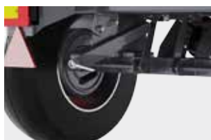
Parking handbrake with crank
