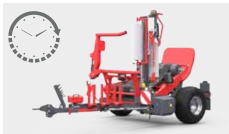
Wrapping with two rolls allows for reducing the required table rotations by half and speeding up the work pace
