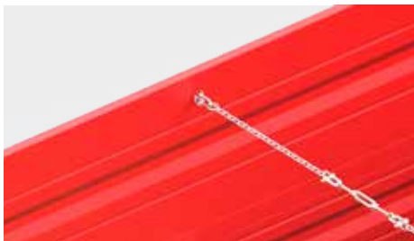
Binding chain - stiffens the cargo space walls
