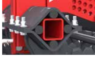
Rubber shock absorbers prevent permanent deformation of the STRENX arm
