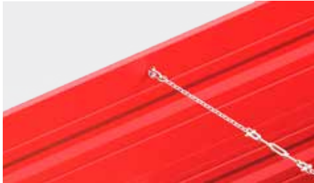
Binding chain - stiffens the cargo space walls
