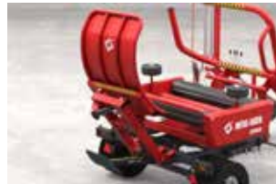
Hydraulic Bale Tipper - A mechanical device for gently unloading a wrapped bale and placing it on the ground
