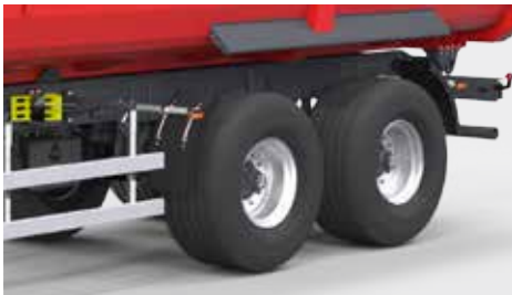
As standard, 560/60-R22.5 tires (RADIAL tires - reinforced tire construction).
