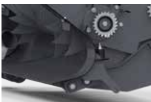
Hydraulically lowerable rotor floor - in case of blockages, facilitates the removal of obstructing material
