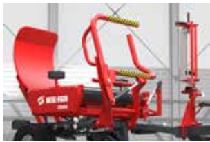
Loading arm - designed for picking up compressed bales of grass, hay, or other non-woody plants from the ground
