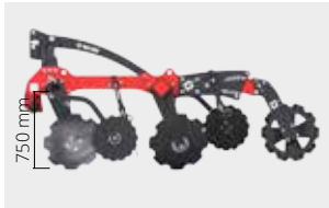
Ground clearance under the frame - 750mm
