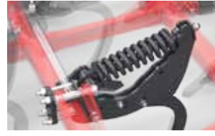
Spring overload protection of working elements
