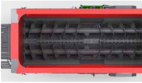
Mixing system based on two horizontal augers located at the bottom of the hopper.
