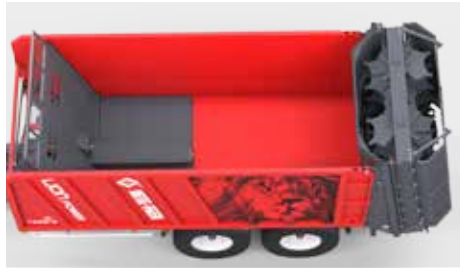
The possibility to convert the trailer into a spreader after installing a horizontal adapter
