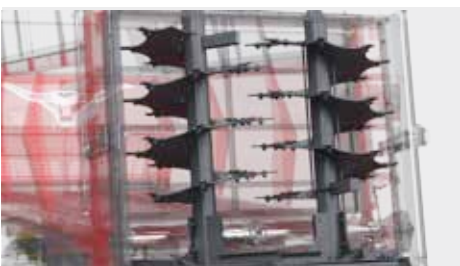
Adapter - blades of elevated durability made from HARDOX
