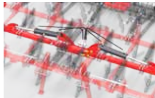
U487 NOVALIS TRIO 420 - hydraulically folding frame
