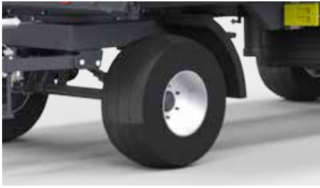
400/60-15.5 tires - the wheels are new as per standard
