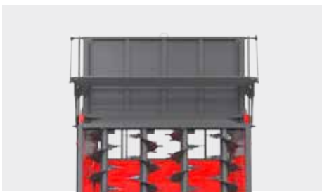
Cover automatically lifted when raising the rear wall (slide) (verti X4)
