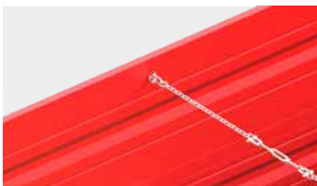
Binding chain - stiffens the cargo space walls
