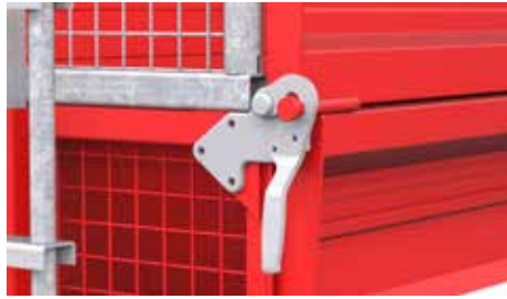
Openable and removable sideboards facilitate easier loading
