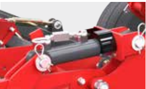
Hydraulic depth adjustment - ensures precise depth adjustment
