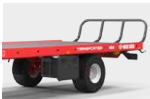
A single-axle chassis has been used, making it easy to maneuver the machine.
