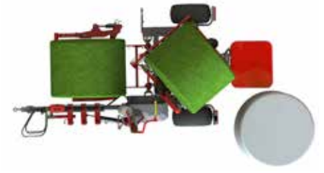
The full cycle time, including loading, wrapping, and unloading of a standard bale with a diameter of 1.2m and using 4 layers of foil, takes approximately 1 minute
