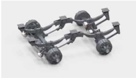
Tandem suspension with a 4-leaf spring.
