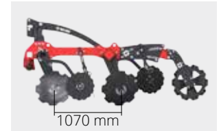
Disc row spacing - 1070 mm
