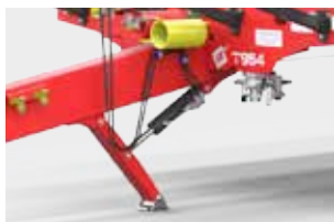
Scissor-hydraulic parking jack
