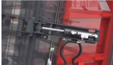
Double hinge for rear flap opening - allows for hydraulic opening of the flap up to 180 degrees
