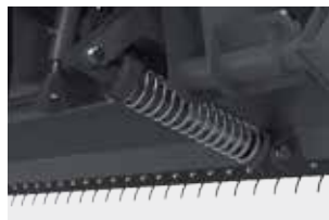
Relief springs – improve ground contour following and reduce the pressure of the copying wheels on the ground
