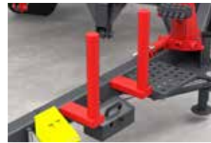
Foil roll holder - a holder for two spare foil rolls is mounted on the drawbar
