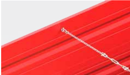
Binding chain - stiffens the cargo space walls
