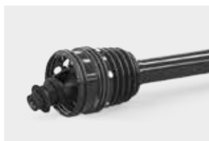
Rotor protection: automatic clutch on the PTO shaft – prevents overloading of the drive system, significantly facilitates the removal of material blockages
