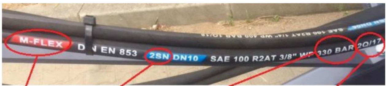
Manufacture Conductor type Max pressure Date of production (in this case, Q2 2017)
