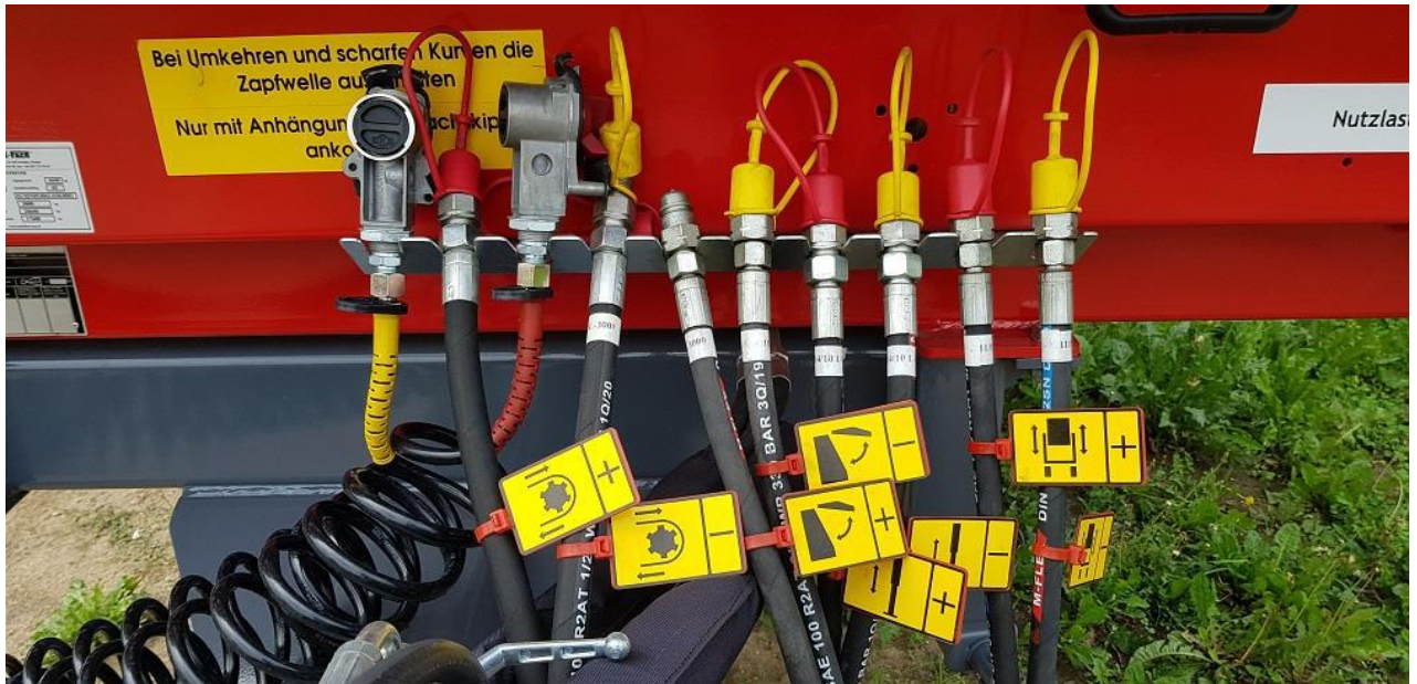
Figure 21 Identification of the hydraulic line couplings with pictograms to facilitate connection of the line to the tractor (standard) – hydraulics without distributor.
