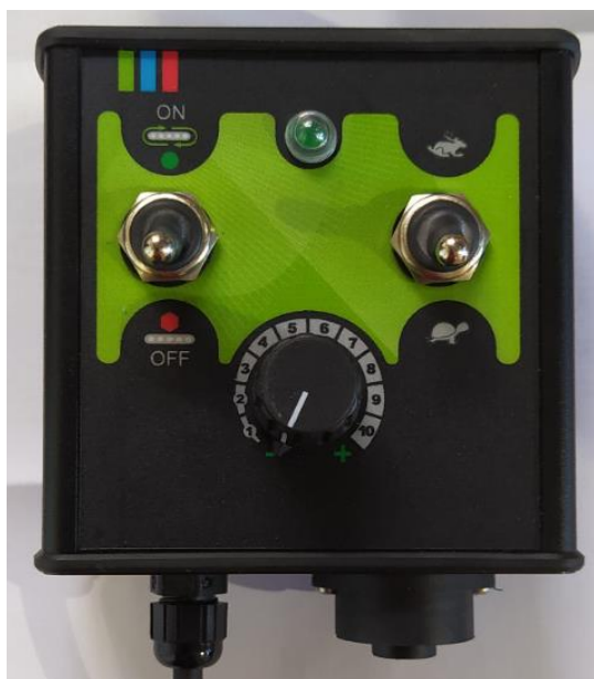
Figure 23 Control panel for adjusting the speed of the floor conveyor.
