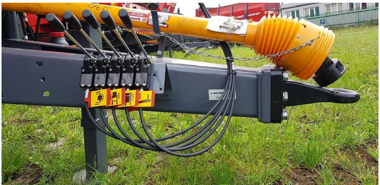
Figure 22 Pictograms for the control levers of the distributor (distributor control is optional).
