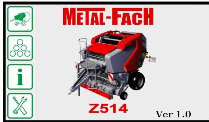
Figure 29. Control Panel – home screen
