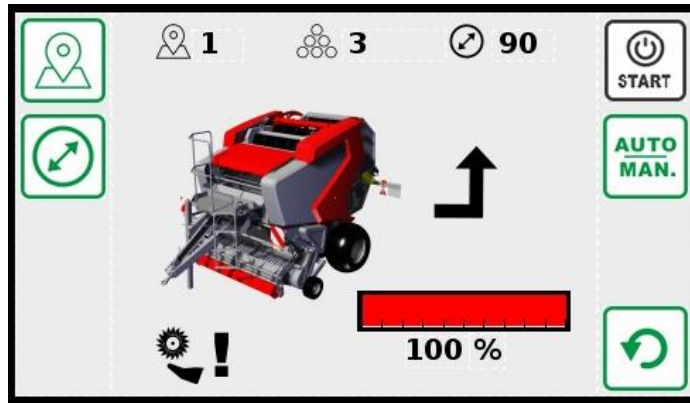
Figure 40. Control panel - opening the rear chamber
