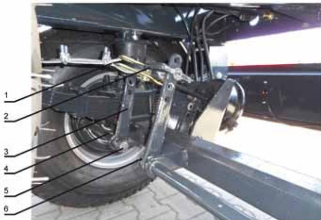
Fig. 10. Braking system components 1 – parking brake cable; 2 – pneumatic cylinder piston rod to expander shaft arm link, 3 – expander shaft arm, 4 – shoe expander shaft; 5 – Seger ring; 6 – expander shaft lever.
