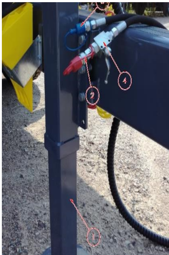
Figure 9. Hydraulic foot. 1- foot, 2 - supply line, 3 – oil-return line, 4 - shut-off valve
