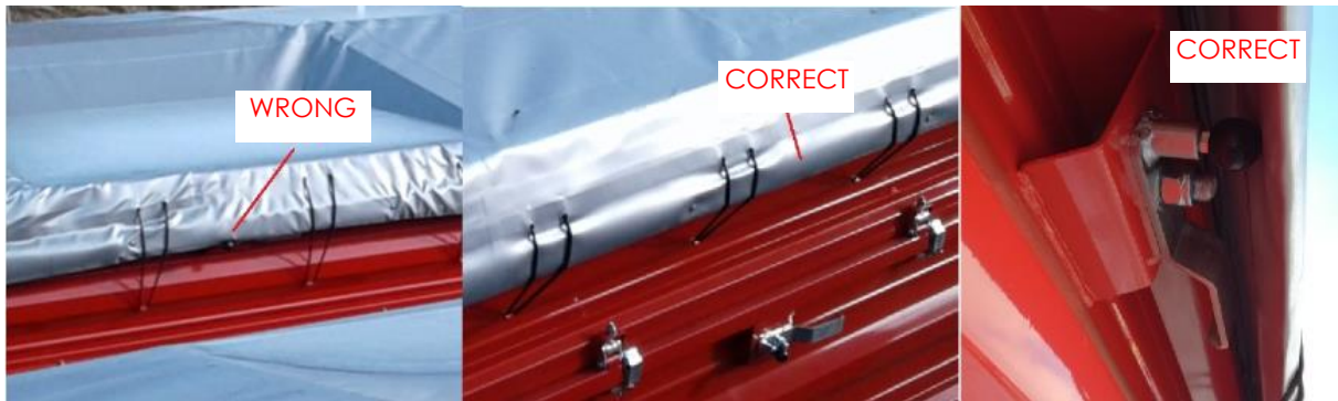
Rysunek 3. Correct tensioning of the canvas cover
