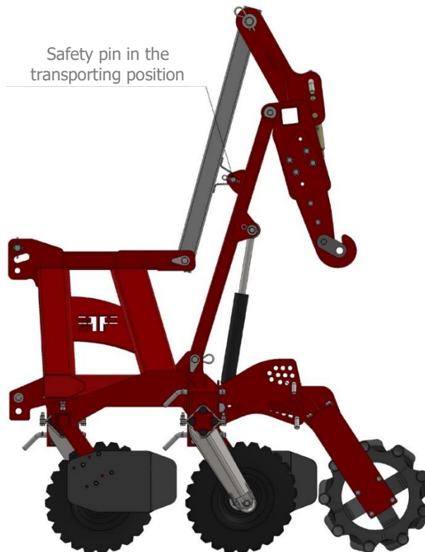
Figure 12. The method for securing the machine in the transporting position
