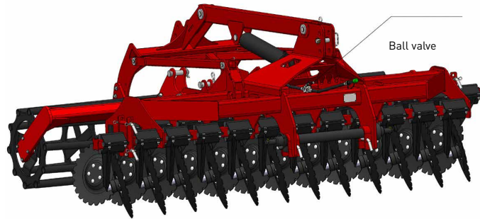
Fig. 11. Securing the cultivator in the transport position
